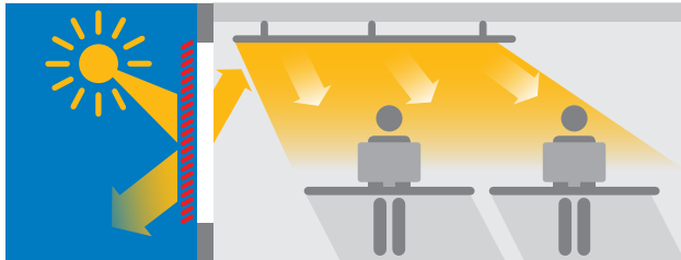
Daylight deflection into the heart of rooms using Atlantic Glow with active solar protection
